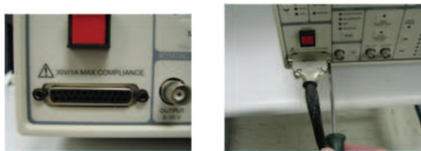
Figure 5: Front panel umbilical connector on EC301. Securing the umbilical cable to the EC301.
