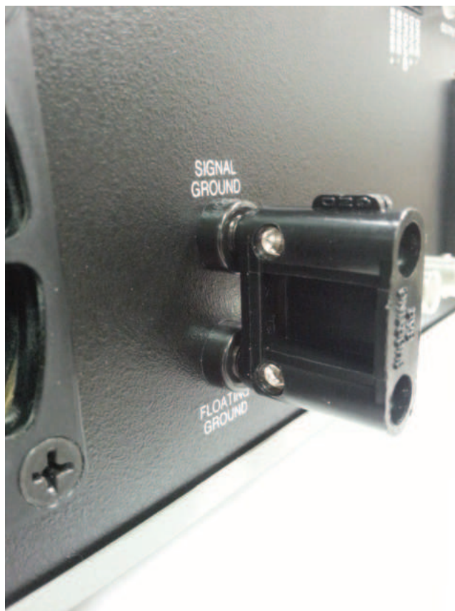
Figure 13: EC301 grounding bar (installed).
