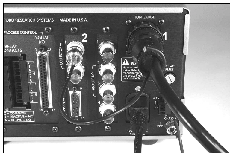
Figure 1-6. Single Ionization Gauge cable connection to the IGC100 controller. 1. 7-pin plug connection to ION GAUGE receptacle, 2. BNC connection to upper COLLECTOR input (labeled '1').
