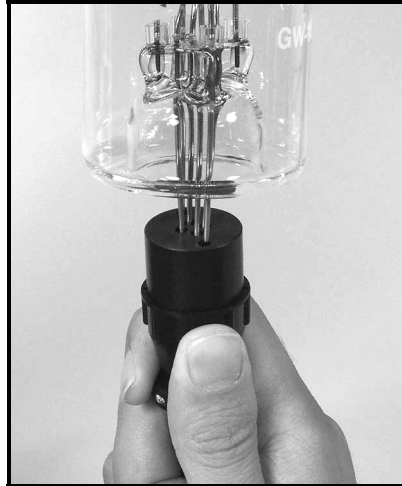
Figure 1-13. O100C2 connection to a dual filament, glass-tubulated, ionization gauge with 6-pin connector header.
