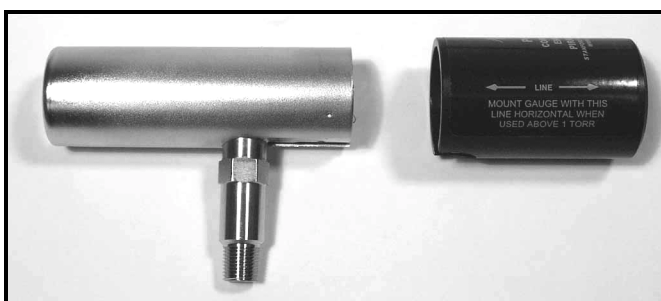
Figure H-6. Side view of the PG105 gauge tube with the detachable plastic connector disconnected.
