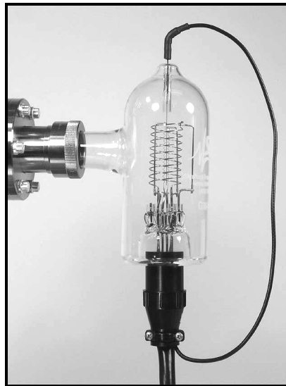
Figure 1-16. Picture of the properly and safely connected glass-tubulated ionization gauge.
