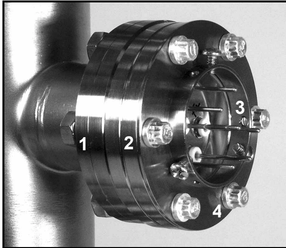
Figure 1-5. The nude ionization gauge attached to the vacuum system (2.75" ConFlat®) Port. 1. Vacuum system port, 2. Gauge feedthrough flange, 3. Metal ring, 4. Bolts (6 places).
