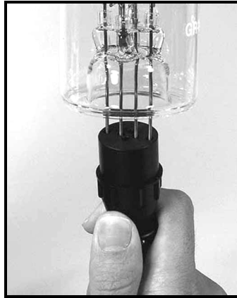
Figure 1-8. O100C1 connection to a single filament, glass-tubulated, ionization gauge with 4-pin header configuration.
