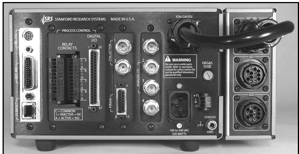
Figure L-5. Connect the IGC100 Ionization Gauge port to the O100IG Box.
