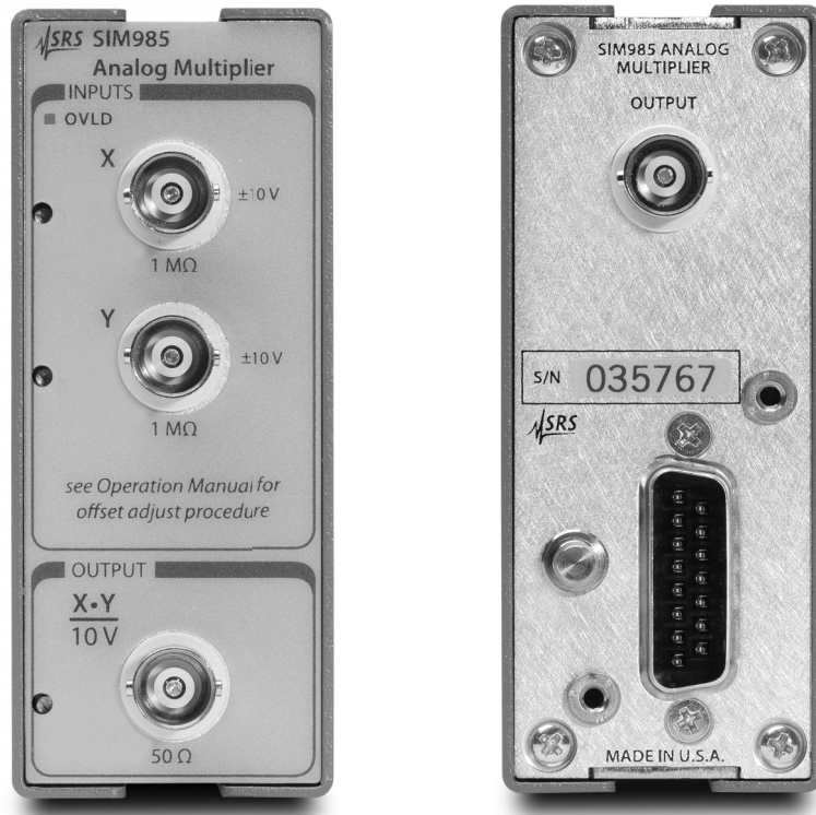
Figure 1.1: The SIM985 front and rear panels.
