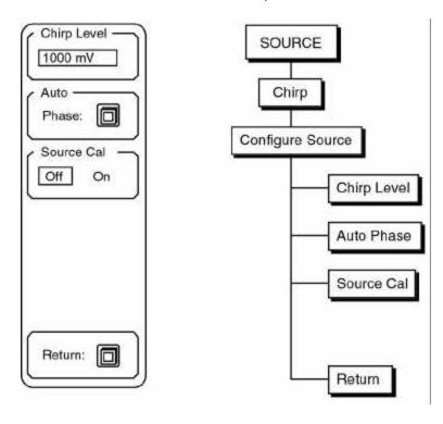
The Chirp source provides an equal amplitude sine wave at each bin of the measurement span. The phases of each sine wave are arranged so that they do not add in phase and the output does not peak. The chirp is EXACTLY periodic over a time record and requires no window. Because of cancellation, the amplitude of each sine wave is NOT constant over the time record. Windowing the time record actually removes necessary spectral information. **USE THE UNIFORM WINDOW WITH THE CHIRP SOURCE.**
