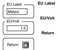
Pressing this key activates the EU Label entry field. Use the ALT keys to enter a name for the engineering units.
