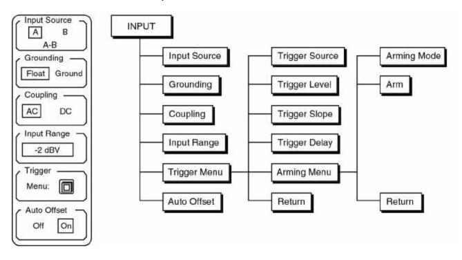
The Input Source key selects the front end signal input configuration. The input amplifier can be single-ended (A) or differential (A-B). In general, when looking at very small signals, connect A to the signal source and B to the signal source ground and use A-B. In this case, make sure that the two input cables do not encompass any loop area (twist them together or run them side by side).
