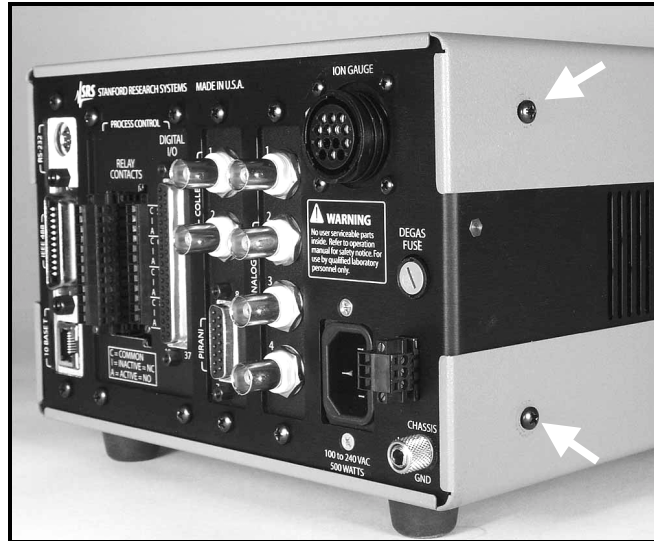
Figure L-2. Remove of the top and bottom cover screws from the back end of the left side of the IGC100.
