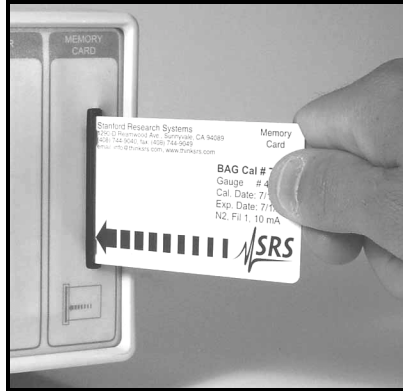
Figure 6-4. Insert the card into the controller.
