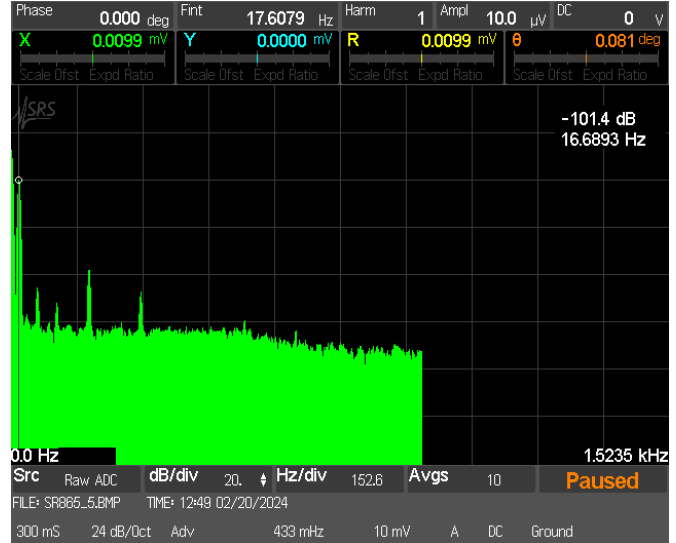
Figure 4: FFT of input signal to SR860. The cursor highlights the signal at the drive frequency. The 60 Hz mains pickup and higher harmonics of 60 Hz can also be seen. These frequencies should be avoided.
