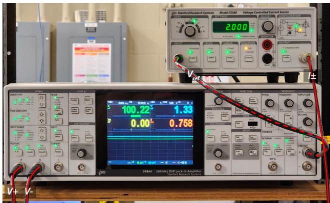
(a) Configuration of SR860 and CS580 for four-point resistivity measurement. The Sine Out ( V_{out} ) from the lock-in is passed to the input of the voltage controlled current source. Current is delivered to the sample's I+ and I- leads with a triax cable ( I\pm ). The V+ and V- terminals are connected to the lock-in voltage inputs A and B, respectively.
